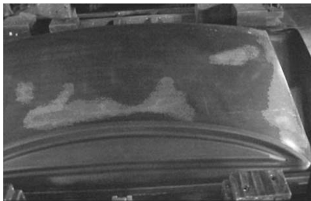
Fig. 4 QPF die used at GM on Oldsmobile Aurora decklid. Oxide layer variation across the tool is observed visually. The lighter regions have a thinner oxide layer and show increased aluminum buildup and galling.
